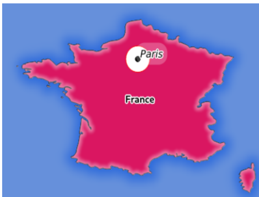
Fig. 3.3: Server response to a GetMap request with FILTER parameter
