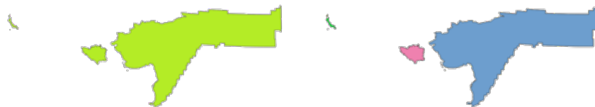
Fig. 28.93: Left the multipart source layer and right the single part output result
