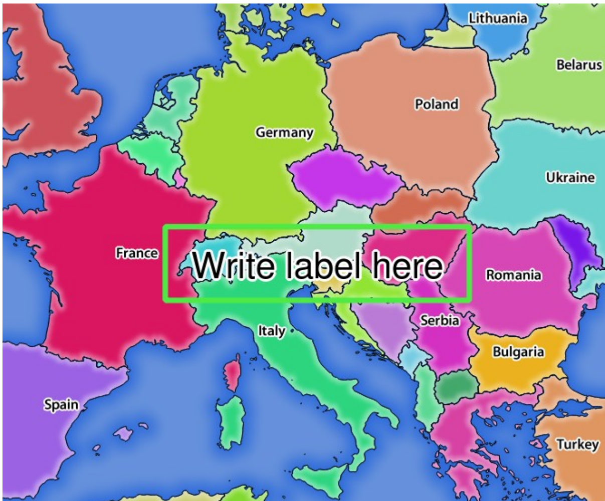
Figura3.22: Server response to a GetMap request with redlining parameters
