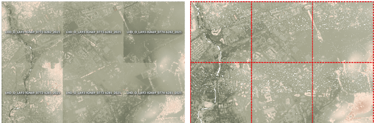
Figura28.13: Generating Virtual Point Cloud with overview from a set of point cloud tiles
