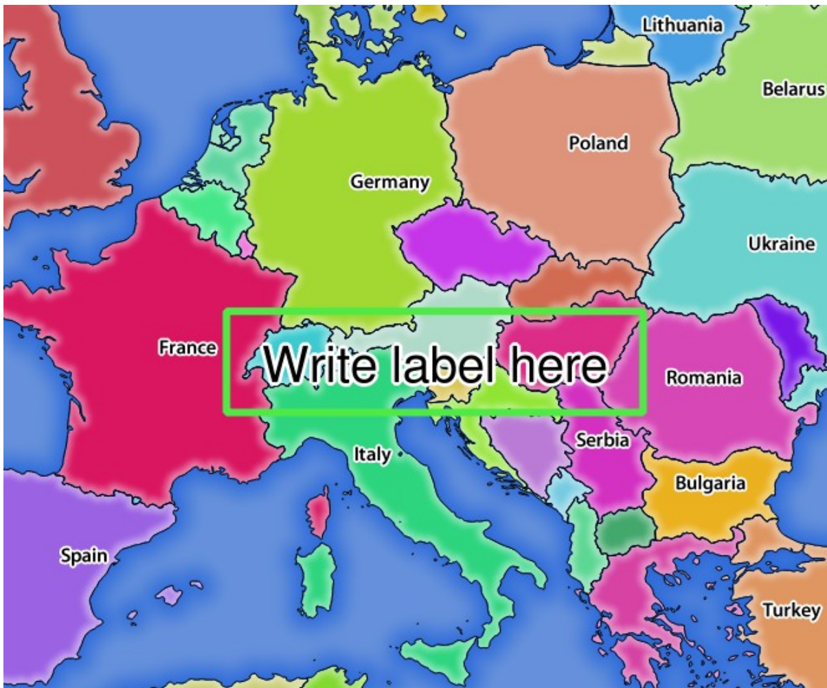
Abb. 3.22: Server response to a GetMap request with redlining parameters
