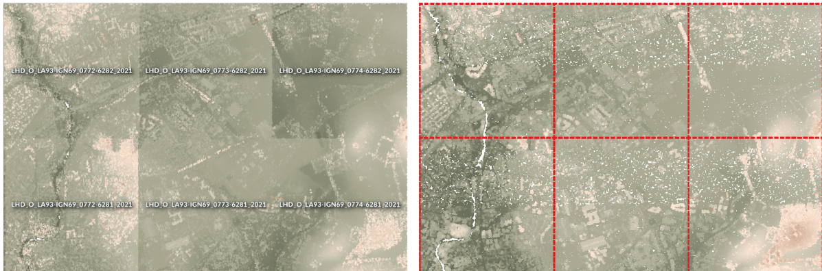
Abb. 28.13: Generating Virtual Point Cloud with overview from a set of point cloud tiles
