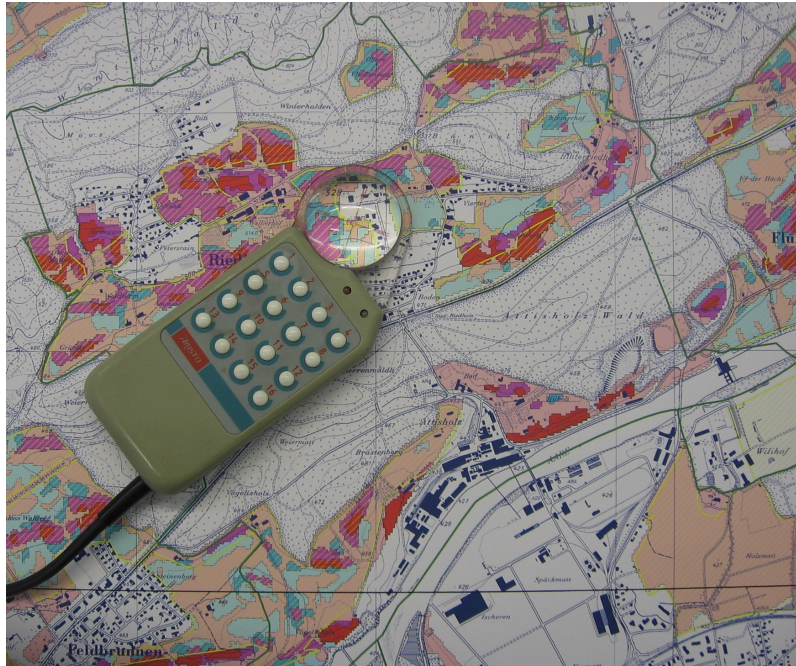
图 5.8: A digitising table and puck are used by GIS professionals when they want to digitise features from existing maps.
