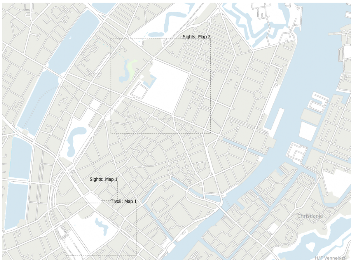
图 11.11: Example of layout extents displayed in a QGIS project with two print layouts. The print layout named 'Sights' contains two map items, while the other print layout contains one map item.
