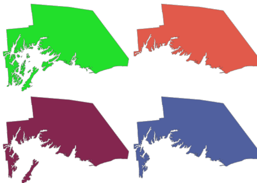
Рис. 28.88: Clockwise from top left: original multipart feature, one, two and three biggest parts kept
