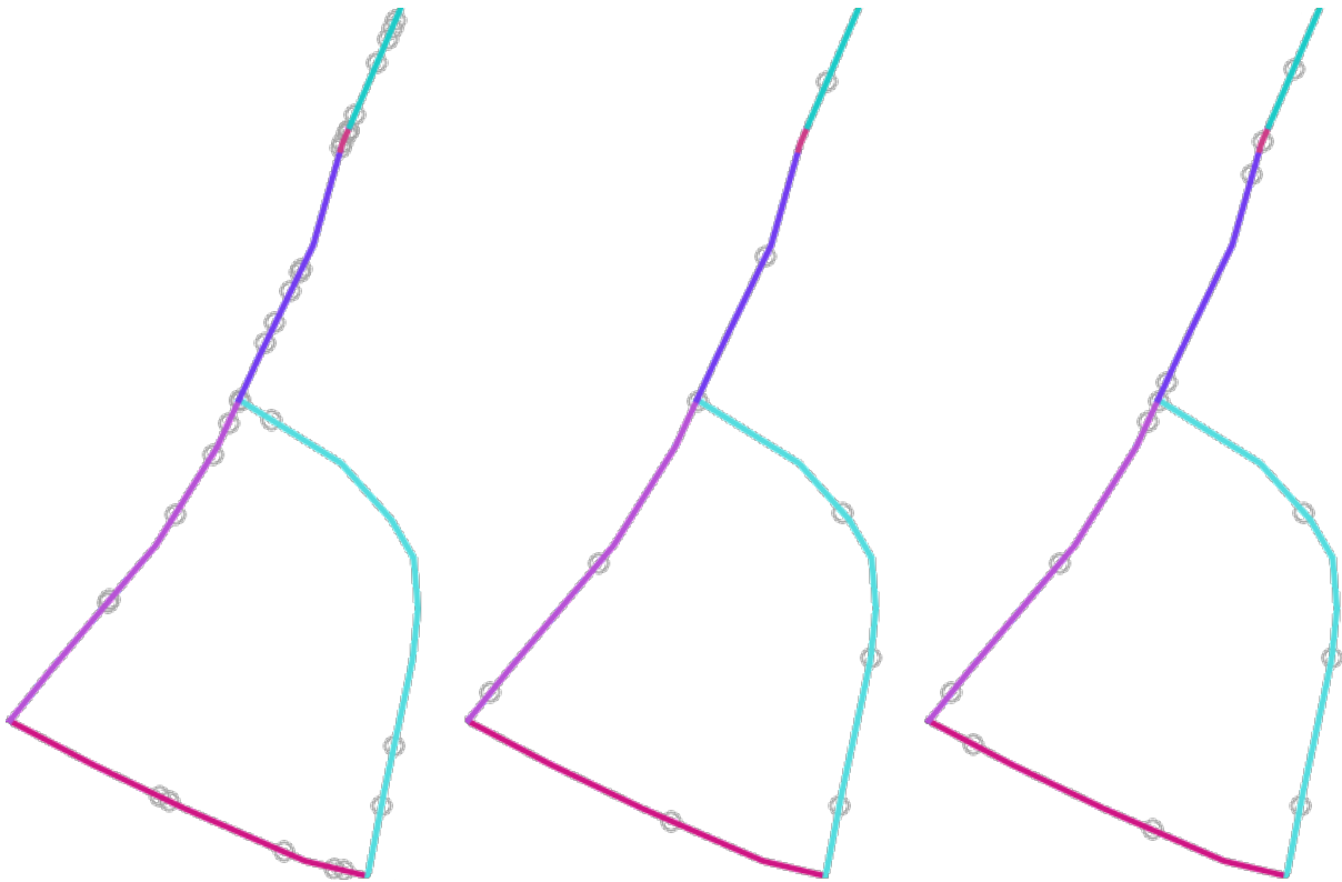
Fig. 28.53: Five points per line feature, left : min. distances = 0, middle : min.distances != 0, right : min. distance != 0, global min. distance = 0
