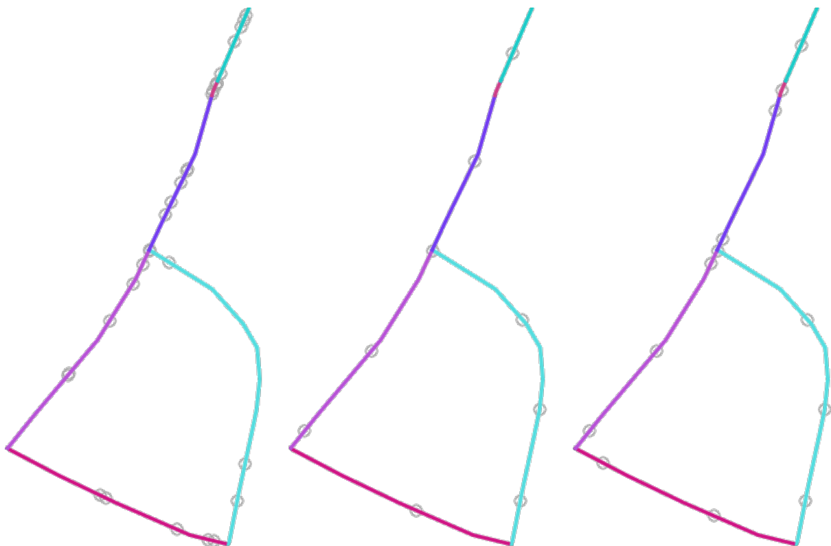
Figura28.53: Five points per line feature, left : min. distances = 0, middle : min.distances != 0, right : min. distance != 0, global min. distance = 0
