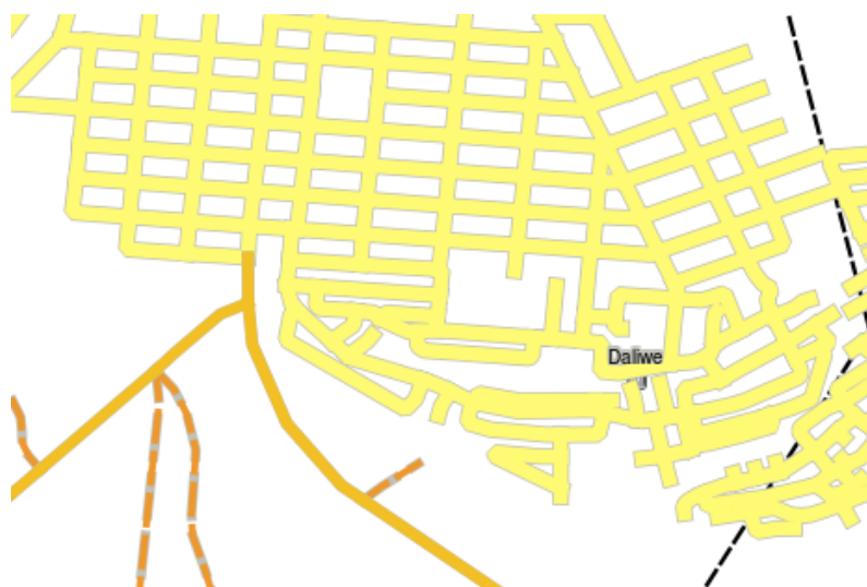
4.14 Fig. : A roads vector layer symbolised using a unique value per road type.
