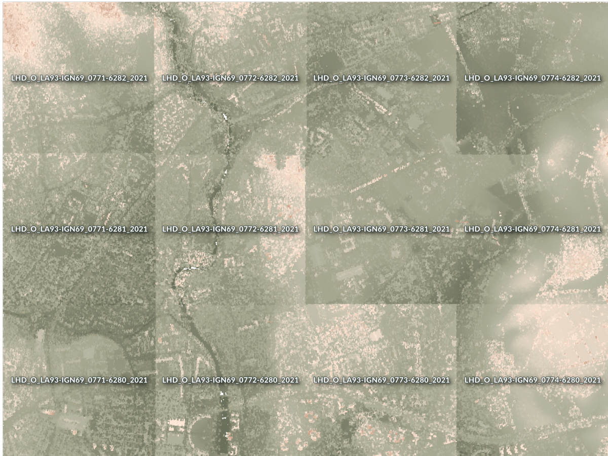
Fig. 20.12: Individual point cloud tiles loaded, with artefacts on edges
