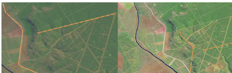
Abb. 5.9: The importance of using properly georeferenced raster images for heads-up digitising. On the left we can see the image is properly georegistered and the road features (in orange) overlap perfectly. If the image is poorly georeferenced (as shown on the right) the features will not be well aligned. Worse still, if the image on the right is used as a reference when capturing new features, the newly captured data will be inaccurate!
