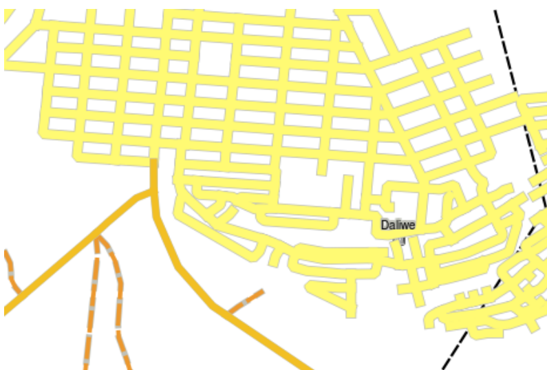
Obr. 4.14: A roads vector layer symbolised using a unique value per road type.
